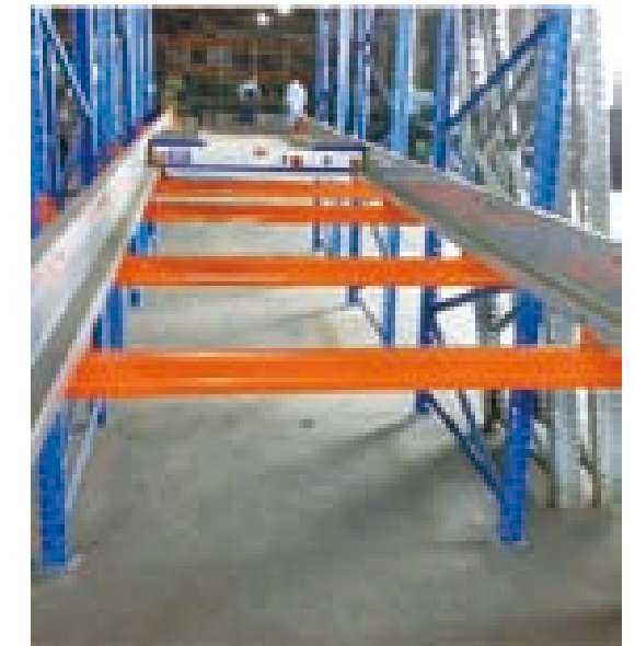
Shuttle car can move the shelves from the depth of the tray to the front, use the forklift to take down the goods.
